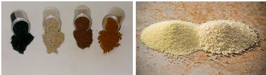
Figure 8: Grinding media used in IsaMill™ applications; in the left hand side photograph samples of furnace slag ex Mt Isa, Colorado River sand, screened ore particles and steel shot and in the right hand side photograph two samples of ceramic media
