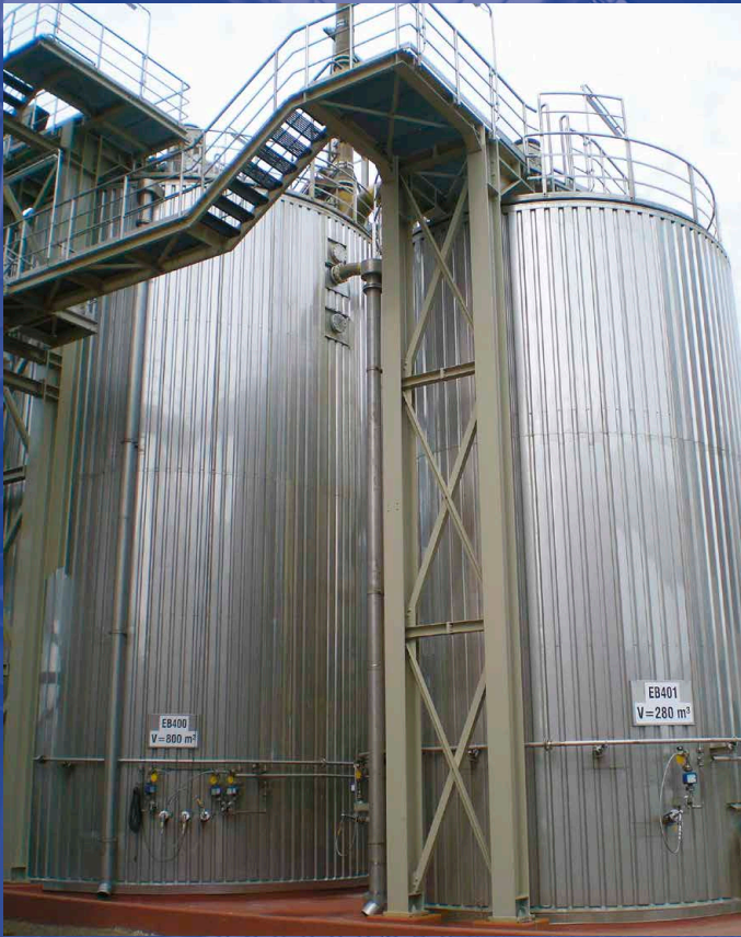
Figure 6: Albion Process™ Leach Reactor
