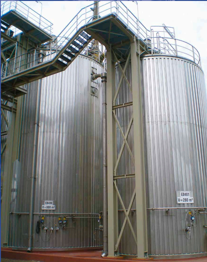
Figure 6: Albion Process™ Leach Reactor
