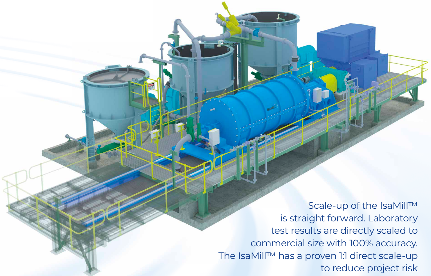
Figure 4: IsaMill™ Grinding Plant Layout
