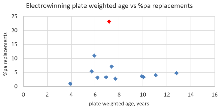
Figure 2. Electrowinning Operating Plate Age and Plate Replacement Rate per Annum
